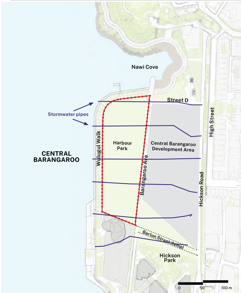
Figure 16: Stormwater drains diagram
