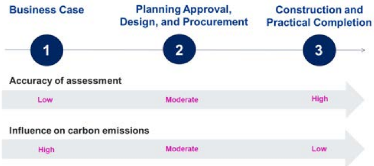
Figure 4.1 Accuracy of measurement and ability to influence carbon emissions at each measurement stage (adapted from PAS2080:2023 s7.1 Figure 7)
