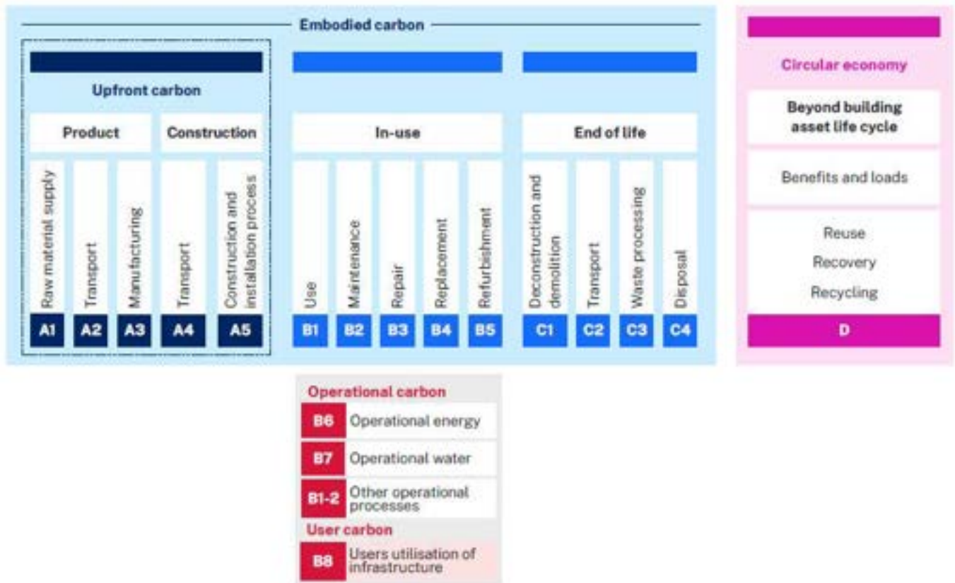
Figure 3.1 Sources of whole life carbon emission and illustration of definitions use in this document (adapted from PAS2080:2023 and modules in EN 17472:2022)
